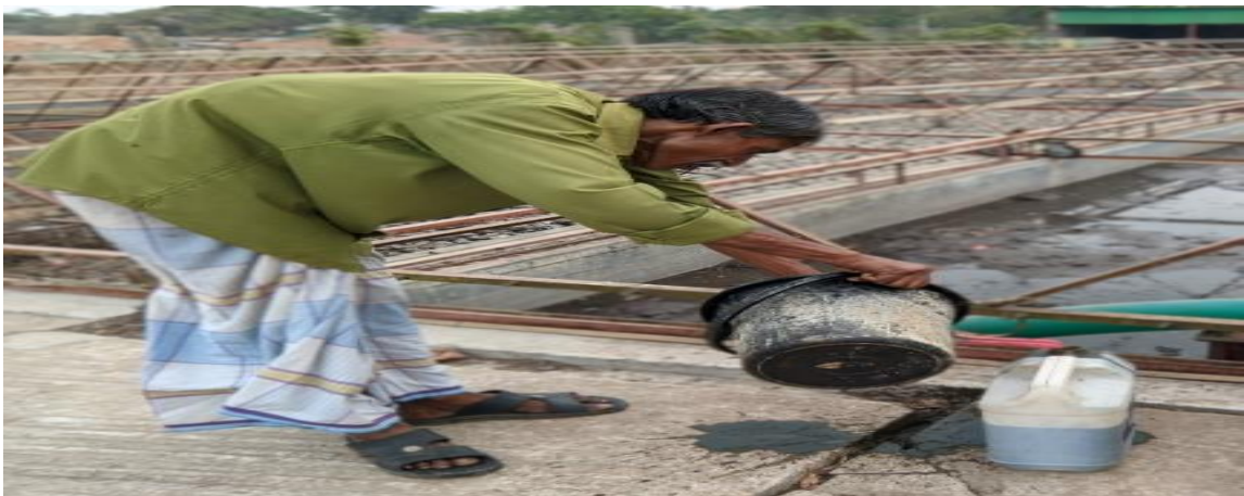
Figure B-1: Faecal Sludge Collection from FSTP, Faridpur
